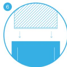
Insert the replacement filter into the unit.
