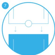
Firmly press the top of the unit onto the replacement filter until you hear a click.
